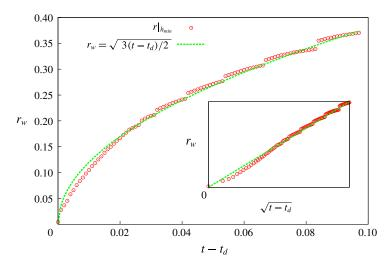
FIGURE 5. (Colour online) Radius  $r_w$ , defined as the radius of minimal height as a function of time  $t-t_d$ , where  $t_d=0.102$  is the time at which the dimple beneath the drop appears, for  $\alpha=0.001$  and m=0.1. The inset shows the relation between  $r_w$  and  $\sqrt{t-t_d}$ . Symbols denote the temporal evolution of the r-coordinate of the  $h_{min}$  point and the dashed curve represents the law  $r_w=\sqrt{3(t-t_d)/2}$ .
