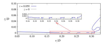
FIGURE 6. (Colour online) The expanding lamella after bubble entrapment (t = 0.059) for the same parameters as in figure 5. The liquid–gas interface is drawn while the solid surface is the dashed line plotted at z = 0. Small bubbles are entrapped within the wetted area due to the rapid expansion of the lamella, as displayed in the inset that shows a zoom of the wetted area.
