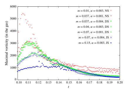
FIGURE 14. (Colour online) Evolution of maximal vorticity in the gas as a function of time for different viscosity ratios ranging from m = 0.01 to m = 0.15 and  $\alpha = 0.001$  to  $\alpha =$ 0.004, covering the different splash and spreading regimes. NS represents non-splashing spreading, DS represents the detachment-splash regime and JS the jet-splash behaviour.
