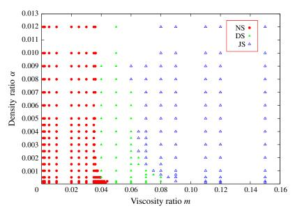
FIGURE 13. (Colour online) Phase diagram of the impact outcome concerning the splashing dynamics. NS represents non-splashing spreading, DS represents the detachment-splash regime and JS the jet-splash behaviour.
