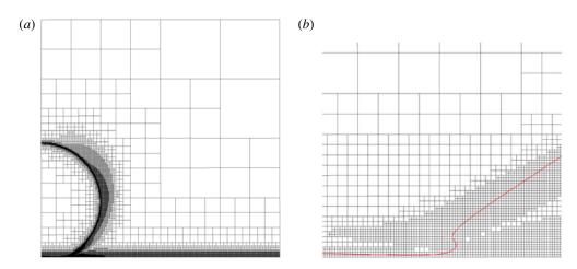
FIGURE 3. (Colour online) Snapshots of the adaptive mesh refinement at two different instants of the impact: (a) just before impact where most of the refinement is concentrated on the interface and solid surface, and (b) a zoom after the impact when a layer of liquid is skating above the solid surface, the red curve representing the interface.
