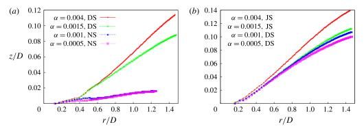
FIGURE 12. (Colour online) Position evolution of the rim of the thin liquid sheet on varying the density ratio  $\alpha = 0.0005, 0.001, 0.0015, 0.004$  with a constant viscosity ratio: (a) m = 0.037 and (b) m = 0.07. NS represents non-splashing spreading, DS represents the detachment-splash regime and JS the jet-splash behaviour. The local minimum observed in (a) around  $r/D \sim 0.6$  for  $\alpha = 0.001$  corresponds to the formation of a liquid rim on the spreading lamella.
