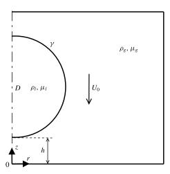
FIGURE 2. Calculation domain. The domain is constituted of a square. A semi-circular droplet of diameter D, density  $\rho_l$  and viscosity  $\mu_l$  falls from a height h with an initial velocity  $U_0$ . The surrounding gas has a density  $\rho_g$ , a viscosity  $\mu_g$  and a surface tension  $\gamma$ . The bottom boundary (z=0) is considered as a solid substrate with no-slip condition and a contact angle  $\theta=90^\circ$  is defined.
