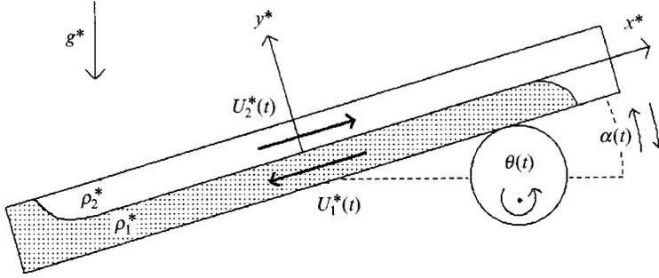
FIGURE 1. Experimental set-up: a tank filled with two fluids of density  $\rho_1^*$  and  $\rho_2^*$  is inclined at an angle  $\alpha_m$  and brought back to its horizontal position in a single rotation of the cam  $0 < \theta \leq 2\pi$ .
