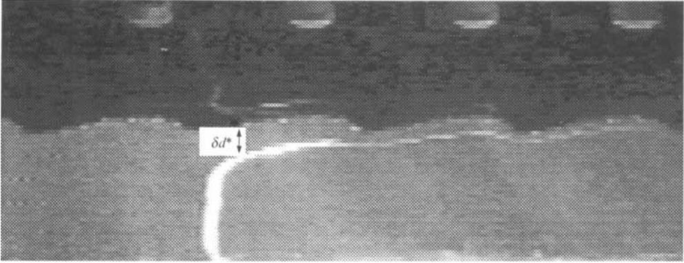
FIGURE 8. Visualization of velocity profile in lower fluid. A vertical dye line is deposited immediately before tilting the tank and its subsequent deformation is recorded. The thickness  $\delta d^*(t^*)$  is determined as the maximum slope thickness of the retrieved profile. Fluid set 2,  $\Delta U_m^* = 14 \text{ cm s}^{-1}$ ,  $\lambda_f^* = 3 \text{ cm}$ ,  $t^* = 2.5 \text{ s}$ .
