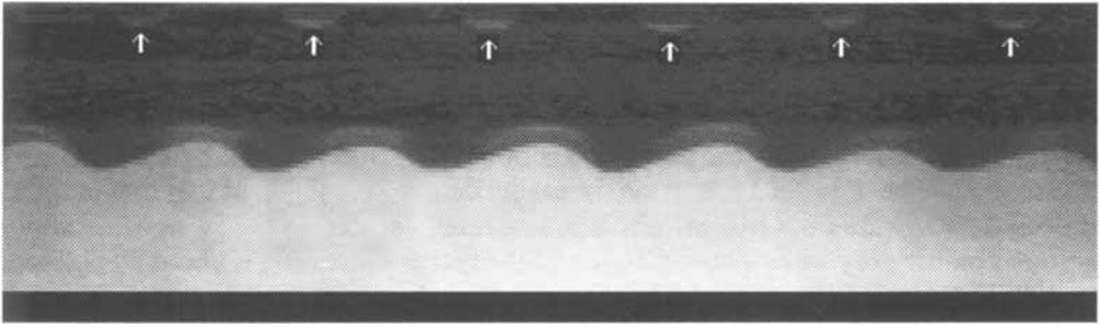
FIGURE 2. Interface deformation 2 s after the onset of instability. Fluid set 2,  $\Delta U_m^* = 16 \text{ cm s}^{-1}$ ,  $\lambda_f^* = 3.7 \text{ cm}$ ; note the location of the periodically distributed obstacles at the top boundary as indicated by the arrows.
