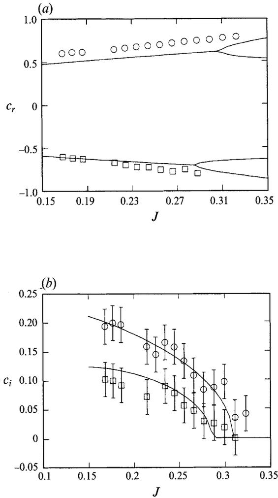
FIGURE 19. Variations of (a) the real part  $c_r$  and (b) imaginary part  $c_i$  of the complex phase velocity as a function of the Richardson number  $J$  for asymmetric velocity profile. The wavenumber is fixed at  $k = 0.51$ . Continuous curves, theoretical predictions;  $\circ$ , experimental data points for right-moving wave;  $\square$ , experimental data points for left-moving wave. Fluid set 3,  $d = 1.4$ ,  $\beta = -0.09$ .
