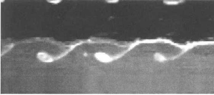
FIGURE 11. Flow visualization of vortex train in lower fluid obtained by dropping fluorescein dye on the interface prior to tilting the tank. Holmboe wave regime. Fluid set 2,  $\Delta U_m^* = 12 \text{ cm s}^{-1}$ ,  $\lambda_f^* = 3 \text{ cm}$ ,  $t^* = 2 \text{ s}$ .
