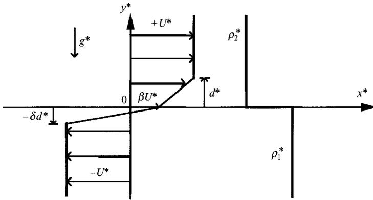
FIGURE 4. Sketch of basic flow for the linear stability analysis of §4.
