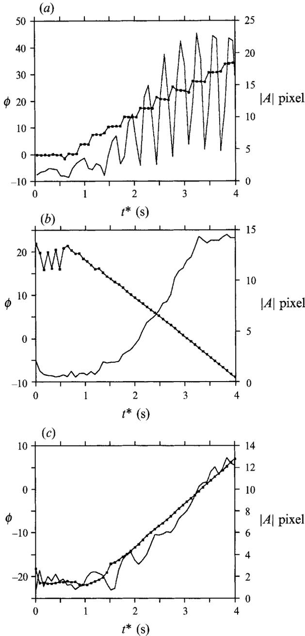
FIGURE 15. Illustration of the procedure used to extract the phase velocity  $c_r$  and growth factor  $c_i$  from the complex amplitude  $A(t)$  at the forcing wavenumber. Fluid set 2,  $\Delta U_m^* = 14 \text{ cm s}^{-1}$ ,  $\lambda_f^* = 3.7 \text{ cm}$ . —, Amplitude  $|A(t)|$ ; ■, phase  $\phi(t)$ . (a) Amplitude and phase variations of total forcing wavenumber component; (b) amplitude and phase variations of left-running wave; (c) amplitude and phase variations of right-running wave.
