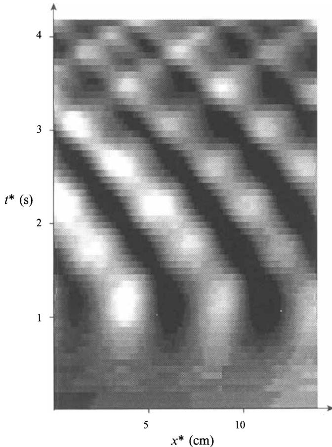
FIGURE 3. Spatio-temporal  $x^*-t^*$  diagram of interface deformation. Fluid set 1,  $\Delta U_m^* = 24 \text{ cm s}^{-1}$ ,  $\lambda_f^* = 5 \text{ cm}$ ; darker (lighter) regions indicate the crest (troughs) of the interface deformation. The tube is brought back to its horizontal position at  $t^* = 1 \text{ s}$ .
