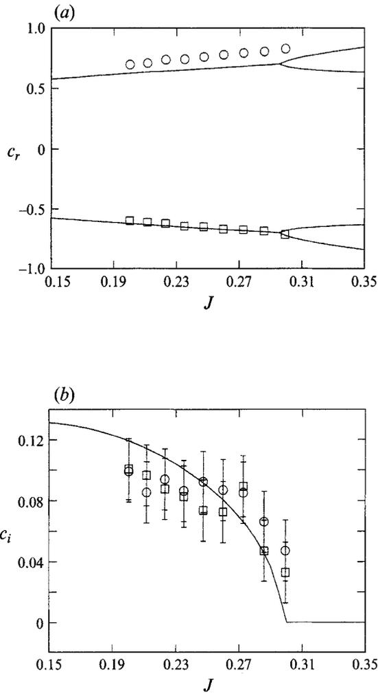
FIGURE 14. Variations of (a) the real part  $c_r$  and (b) imaginary part  $c_i$  of the complex phase velocity as a function of the Richardson number  $J$  for symmetric velocity profile. The wavenumber is fixed at  $k = 0.54$ . Continuous curves, theoretical predictions;  $\circ$ , experimental data points for right-moving wave;  $\square$ , experimental data points for left-moving wave. Fluid set 2,  $d = 1.9$ ,  $\beta = 0$ .
