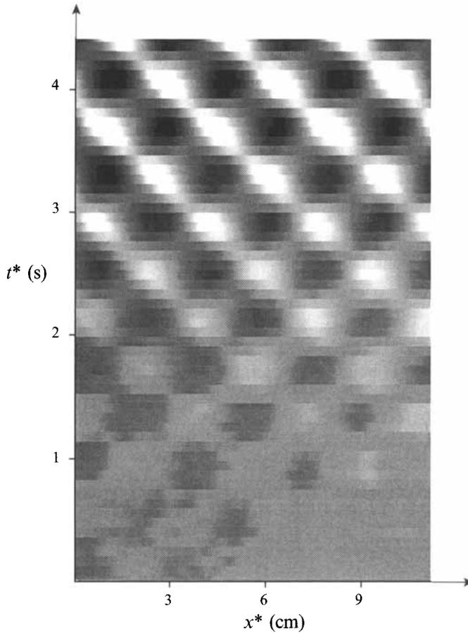
FIGURE 12. Spatio-temporal  $x^*-t^*$  diagram of the interface deformation. Fluid set 2,  $\Delta U_m^* = 14 \text{ cm s}^{-1}$ ,  $\lambda_j^* = 3.7 \text{ cm}$ . The tube is brought back to its horizontal position at  $t^* = 0.72 \text{ s}$ .
