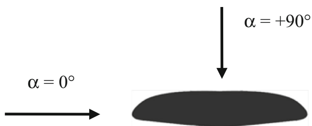
Fig. 5 Definition of the angle of attack on the Aleutian blade paddle
