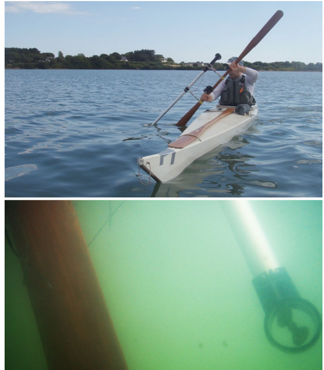
Fig. 4 Views of the flow meter mounted on the paddle
