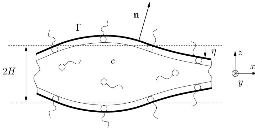
FIGURE 1. Soap film internal structure
