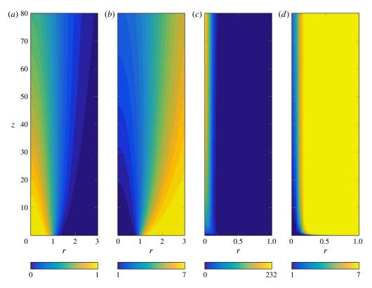
FIGURE 1. (Colour online) Axisymmetric steady base flows obtained for  $Ri = 10^{-4}$  (*a,b*) and for  $Ri = 10^3$  (*c,d*). Axial velocity (*a,c*) and density (*b,d*) are shown in the (*r, z*) plane.
