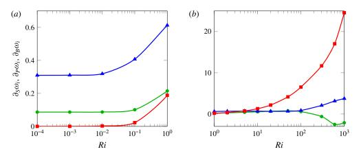
FIGURE 8. (Colour online) Sensitivity of the growth rate with respect to ( $\blacktriangle$ ) shear, ( $\bullet$ ) baroclinic and ( $\blacksquare$ ) buoyancy terms, as functions of the Richardson number, with parameters S = 7 and Re = 200.
