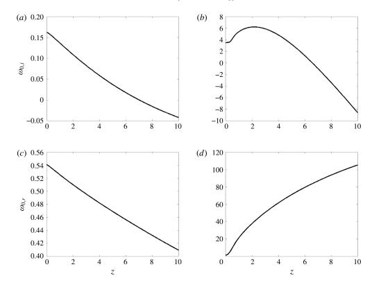
FIGURE 9. Variation of the absolute frequency  $\omega_0$  with streamwise location z for the axisymmetric mode m = 0 and  $Ri = 10^{-4}$  (a,c) and  $Ri = 10^2$  (b,d) at S = 7, Re = 200.
