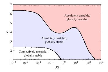
FIGURE 6. (Colour online) Instability regimes in the *S*–*Ri* plane for the axisymmetric mode at Re = 200. The thick line denotes the global stability boundary, and the thin line denotes the boundary between local convective and absolute instability of the inlet profile.
