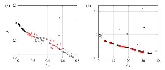
FIGURE 3. (Colour online) Global spectra of axisymmetric perturbations (m = 0), for the two configurations shown in figure 1. (a)  $Ri = 10^{-4}$ , jet case; (b)  $Ri = 10^3$ , plume case. Re = 200 and S = 7 are set identically for both cases. True eigenvalues (O) are compared to their counterparts (+) that are obtained when the buoyancy term in (2.11b) is removed.
