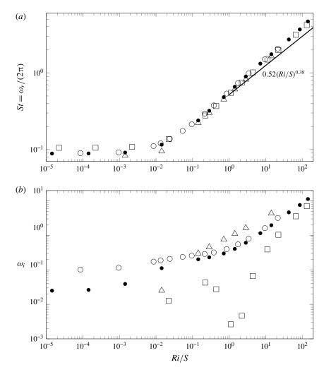
FIGURE 5. (a) Strouhal number and (b) growth rate of the global eigenvalue  $\omega$ , as a function of Ri/S. Legend: (•) Re = 200, S = 7; (○) Re = 500, S = 7; (□) Re = 200, S = 4.5; (△) Re = 200, S = 7, with parabolic inlet velocity profile. All other configurations take the inlet velocity profile (2.8). (----) Power law from the Cetegen & Kasper (1996) experiments, rescaled to match the present definition of Ri.
