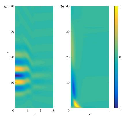
FIGURE 4. (Colour online) Spatial distributions of axial velocity eigenfunctions  $\hat{u}_z$ , corresponding to the most unstable modes of the two respective cases shown in figure 3. (a) Jet at  $Ri = 10^{-4}$ , S = 7 and Re = 200; (b) plume at  $Ri = 10^3$ , S = 7 and Re = 200.
