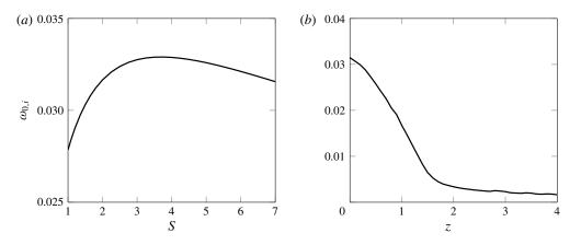
FIGURE 10. Absolute growth rate  $\omega_{0,i}$  of helical perturbations, for Re = 200 and Ri = 1: (*a*) at the inlet, as a function of the density ratio S; (*b*) as a function of z, for S = 7.
