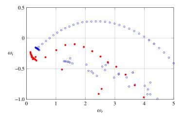
FIGURE 7. (Colour online) Global spectrum of helical perturbations (m = 1), for the configuration S = 7, Ri = 1 and Re = 200. Results from two calculations are shown: (O) without absorbing layer; ( $\bullet$ ) with absorbing layer at z > 30.
