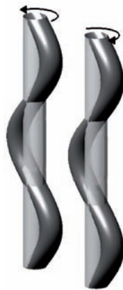
Figure 1.8: Sketch of the zigzag mode of a pair of counter-rotating vortices: the vortices are bended on the vertical. From Billant et al. (2007).
