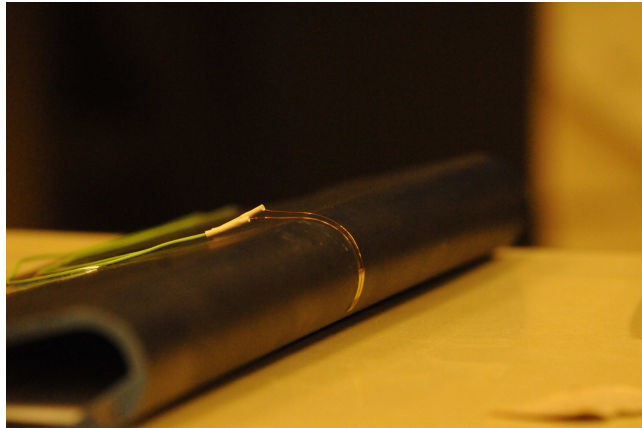
FIG. 13 – Hot-film placement on the airfoil. Bboundary layer perturbations are sensed on the leading edge. The wires are placed on the uncontrolled side.
