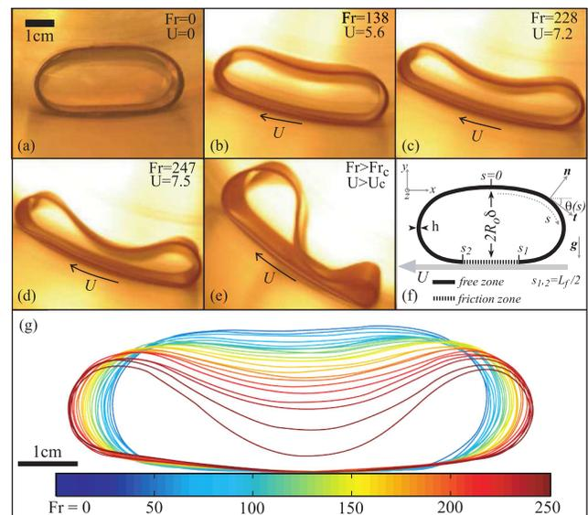
FIG. 1 (color online). A ribbon rolling at different speeds [or Froude number  $Fr = U^2/(gR_0)$ ]: (a)  $Fr = 0$ , (b)  $Fr = 143$ , (c)  $Fr = 236$  (d)  $Fr = 259$ , (e) An unsteady shape observed above the critical touchdown speed. (f) A schematic of the ribbon. (g) Experimentally observed dependence of ribbon shape on Froude number. Ribbon properties:  $E = 0.26$  MPa,  $\rho = 1050$  kg/m<sup>3</sup>,  $h = 1.6$  mm,  $w = 27$  mm.
