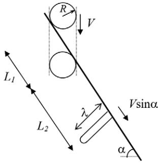
**Fig. 6.** A drop crossing an inclined thin fiber at  $V > V^*$ : the drop first crosses the thread (in a time denoted as  $\tau_1$ ), and then it elongates before breaking (in a time denoted as  $\tau_2$ ). We call  $\ell$  and  $r$  the length and radius of the cylindrical elongated drop at  $t = \tau_2$ .
