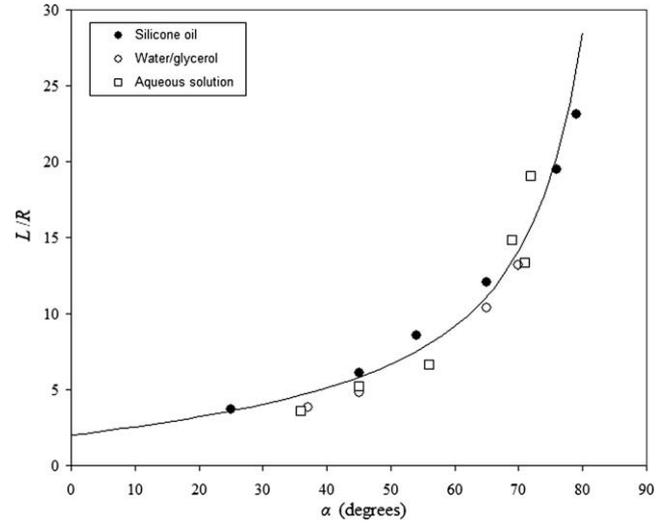
**Fig. 8.** Distance  $L$  on which the drop coats the fiber before detaching ( $V > V^*$ ) normalized by the drop radius  $R$ , as a function of the tilt angle  $\alpha$ , for various liquids on a nylon fiber of radius  $b = 250$   $\mu\text{m}$ . The symbols correspond to different liquids whose characteristics are given in Fig. 3. The solid line is the function  $2/\cos\alpha + 3\tan\alpha$ .
