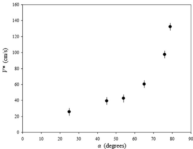
**Fig. 2.** Critical velocity of capture of drops of silicone oil ( $R = 1$  mm,  $\gamma = 20$  mN/m,  $\rho = 915$  kg/m<sup>3</sup> and  $\eta = 5$  mPa s) below which the drops are fully captured by a nylon fiber ( $b = 250$   $\mu$ m), as a function of the tilting angle  $\alpha$  (measured from the horizontal) of the fiber. It is observed that the capture is made much more favorable when inclining the fiber.
