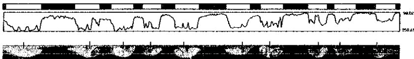
FIG. 10. (a) ( y - z ) view of the streamwise counter-rotating vortices with location of the streaks. (b) Intensity profile taken in (a) along the line. (c) Interpretation: (white) \rightarrow regions of vortex-dominated dynamics; (grey) \rightarrow regions of relative inactivity. ( \rho/h = 0.0571 , R = 190 )
