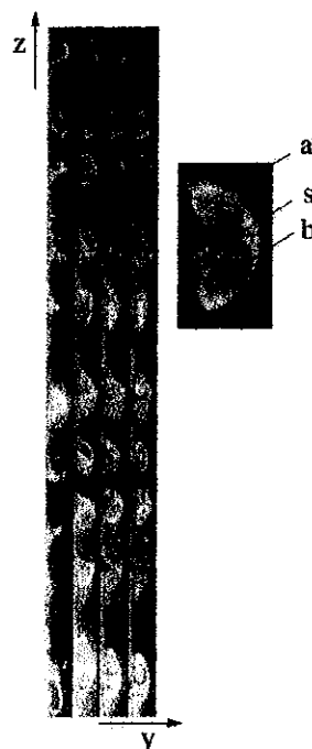
FIG. 8. ( y - z ) view of the streamwise counter-rotating vortices. Four snapshots at a regular interval of 5 s are displayed. Each image shows the whole gap. The insert displays one given structure made of two vortices (a) and (b) inducing the streak (s) between them by the lift-up mechanism. ( \rho/h=0.0571 , R=190 .)
