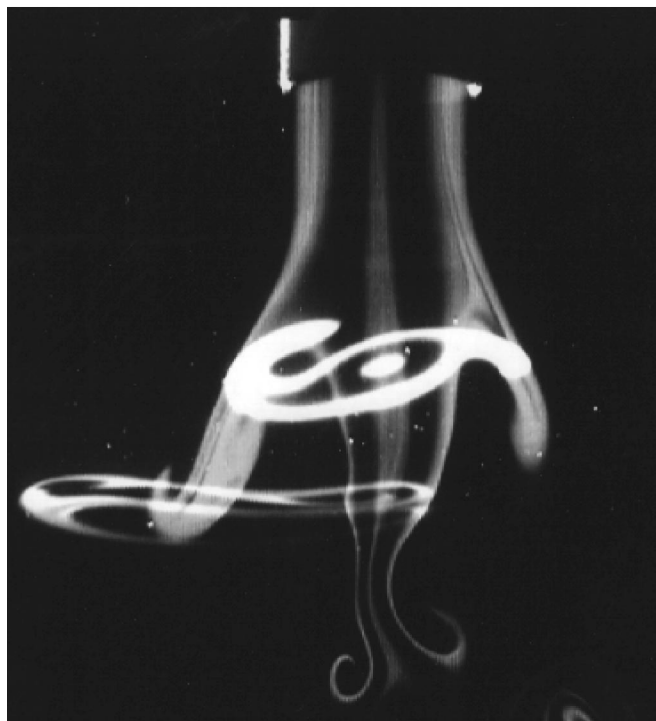
FIG. 22. Flow visualization of the precursor state in the swirling jet experiment of Billant et al. 8 prior to vortex breakdown onset. Overlaid vertical and horizontal laser sheets showing the double helical pattern dominated by |m|=2 .
