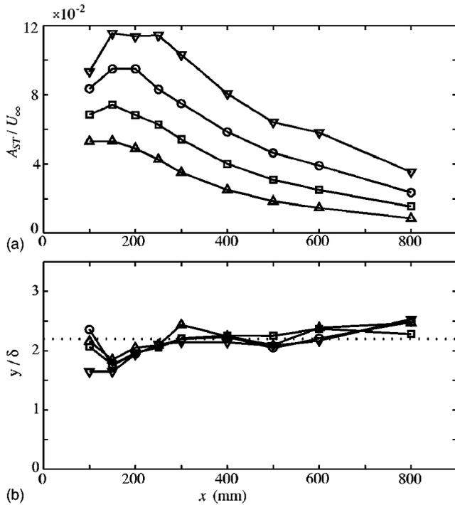
FIG. 6. Streamwise evolution of the streaks: (a) Streak amplitude  $A_{ST}$  vs  $x$  (mm). (b) Wall-normal position of the maximum streak amplitude normalized with the local Blasius length scale  $\delta$ . The symbols ( $\Delta$ ), ( $\square$ ), ( $\circ$ ), and ( $\nabla$ ) correspond to  $U_\infty=5, 6, 7$ , and  $8$  m/s, respectively.
