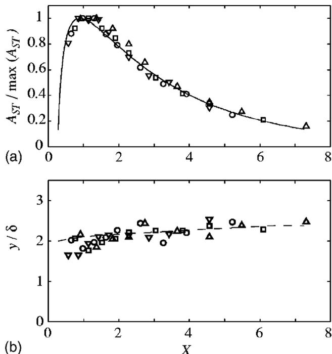
FIG. 11. Comparison between the experimental results for all  $U_\infty$  in Table I and the best fitting to  $U_\infty=7$  m/s obtained using initial vortices confined closer to the wall ( $c=0.78$ ). (a) Wall-normal maximum of the streak amplitude. (b) Wall-normal position of the maximum perturbation.
