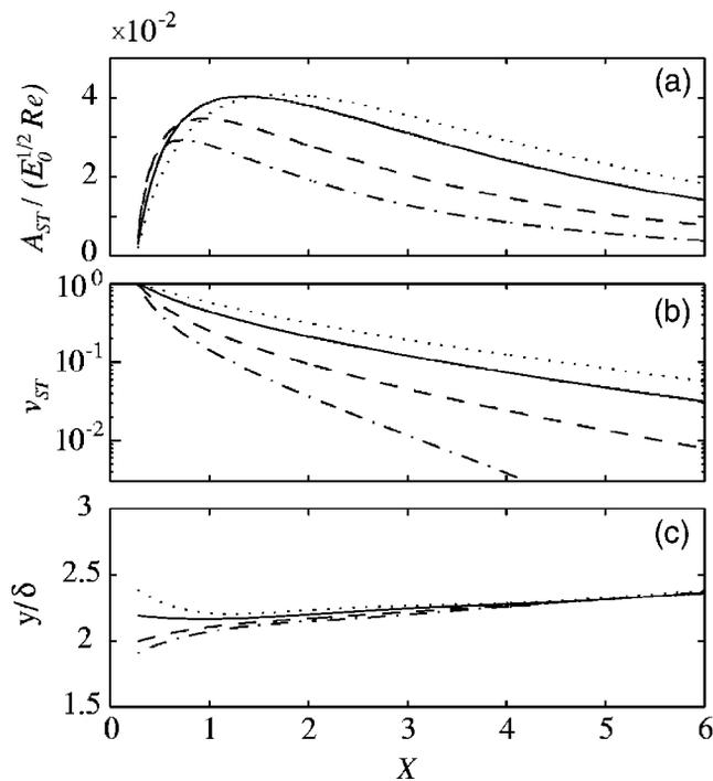
FIG. 10. Streamwise evolution of the streak generated by initial conditions at  $X_0=0.2611$ ,  $\beta_0=0.2299$ . (a) Streamwise velocity amplitude; (b) wall-normal maximum of the wall-normal velocity amplitude; and (c) wall-normal maximum of the streamwise velocity perturbation. Solid line:  $c=1$  (optimal disturbance); dotted line:  $c=1.2$ ; dashed line:  $c=0.8$ ; dash-dotted line:  $c=0.7$ .
