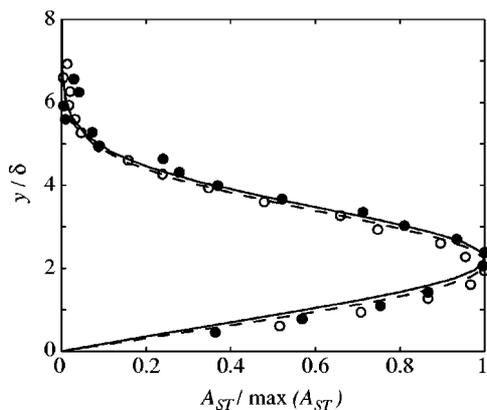
FIG. 12. Wall-normal perturbation profiles at  $x=200$  and  $500$  mm (or  $X=1.31$  and  $3.26$ ) corresponding to unfilled and filled symbols, respectively. Dashed and solid lines are the corresponding theoretical profiles.
