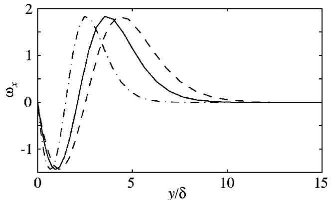
FIG. 9. Wall-normal distribution of the streamwise vorticity of optimal disturbance at  $X_0=0.2611$ ,  $\beta_0=0.2299$  (solid line). Suboptimal initial conditions obtained by stretching or compressing the optimal disturbance by a factor  $c$ . Dashed line:  $c=1.2$ ; dash-dotted line:  $c=0.7$ .
