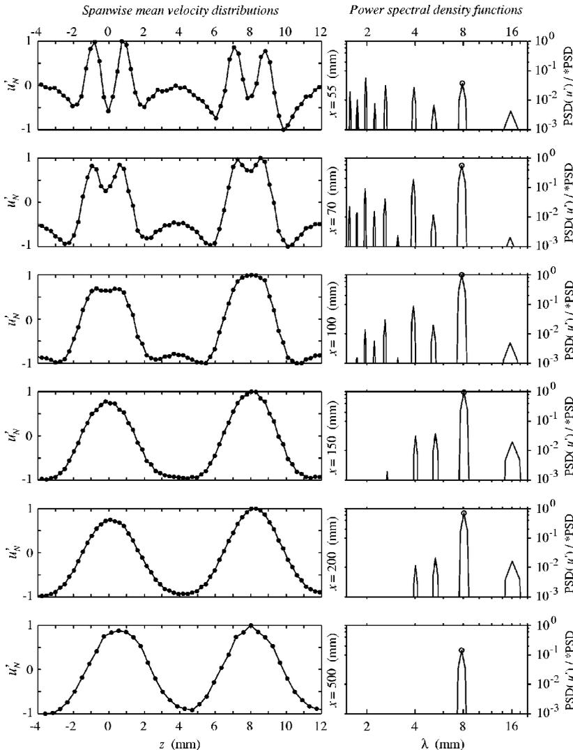
FIG. 4. Streamwise evolution of the mean spanwise velocity profile taken at the wall-normal position corresponding to the disturbance peak. (a) Spanwise velocity distribution normalized to  $\pm 1$ , and (b) spanwise power spectral density function. The normalization is such that  $*PSD$  corresponds to  $\max\{PSD(u')\}$  for all  $x$ .  $U_\infty = 7$  m/s.
