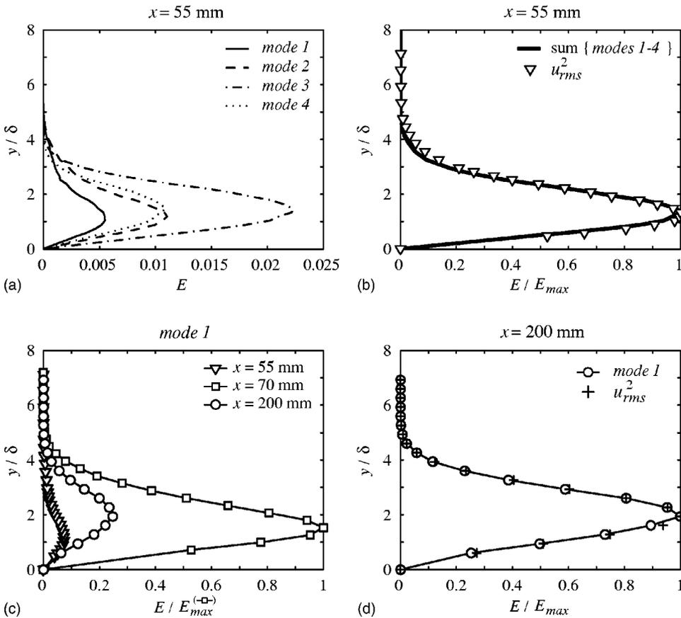
FIG. 5. Decomposed energy mode profiles in the wall-normal direction.  $U_\infty = 7$  m/s. (a) Power spectral density distributions for the fundamental (1) mode  $\lambda_0 = 8$  mm and higher harmonics; (2)  $\lambda_0/2$ , (3)  $\lambda_0/4$ , and (4)  $\lambda_0/5$ . (b) Comparison between the  $u_{rms}^2$  (Fig. 3) and the superposition of all four modes. (c) Fundamental mode for different  $x$  positions. (d) Comparison between the  $u_{rms}^2$  (Fig. 3) and the fundamental mode.
