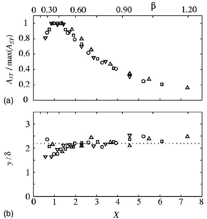
FIG. 7. Streamwise evolution of the streaks: (a) Streak amplitude  $A_{ST}$  normalized to unity vs the boundary layer streamwise coordinate  $X$  and the local spanwise wave number  $\beta=2\pi\delta/\Delta z$ . (b) Wall-normal position of the maximum streak amplitude normalized with the local Blasius length scale  $\delta$ . Symbols are same as in Fig. 6.
