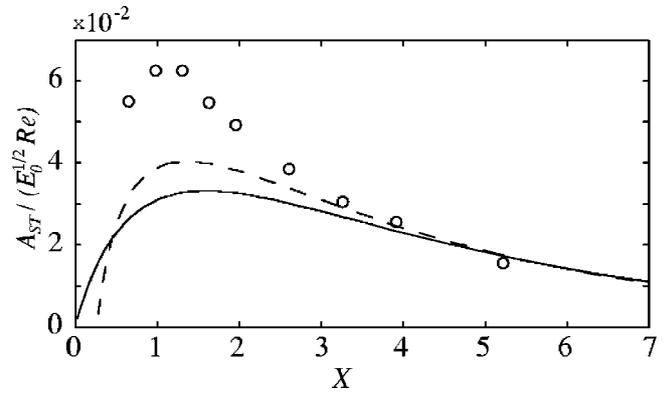
FIG. 8. Streamwise evolution of the wall-normal maximum of the streamwise velocity perturbation of the optimal perturbations introduced at the leading edge (solid line) and at the actual position of the roughness elements  $X_0=0.2611$  (dashed line). The open circles indicate the measured streak amplitude  $A_{ST}$ , scaled to compare the final decay rates.
