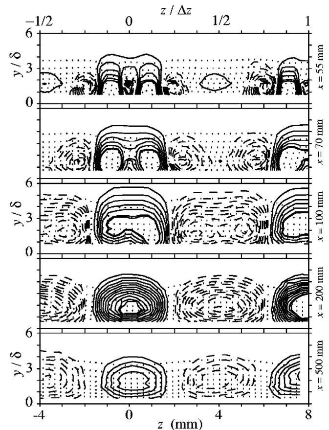
FIG. 2. Streamwise evolution of positive and negative streamwise velocity perturbations (solid and dashed lines, respectively). Dotted contour lines (0.1  $U_\infty$  of increment) correspond to constant streamwise velocity.  $U_\infty = 7$  m/s.
