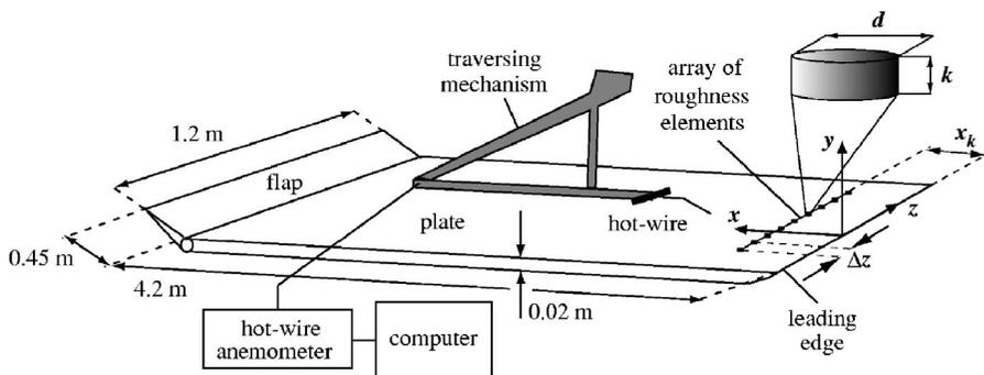
FIG. 1. Schematic of the experimental setup.  $k=780\ \mu\text{m}$ ,  $d=2\ \text{mm}$ ,  $\Delta z=8\ \text{mm}$ , and  $x_k=40\ \text{mm}$ .
