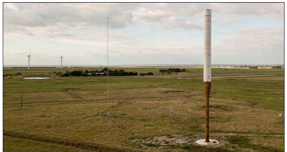
Fig. 1: Experimental chimney in the monitored field (the mast with wind anemometers is slightly visible, see Fig. 2 for details)
