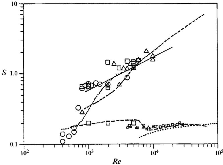
FIGURE 3. Strouhal number as a function of  $Re$ . ..... , Achenbach (1974); -----, Kim & Durbin (1988); —,  $S_{\lambda'}$ . Small symbols correspond to velocity probe measurements and large symbols to values determined from visualizations.  $\circ$ ,  $R = 1.12$  cm;  $\square$ ,  $R = 2.5$  cm;  $\triangle$ ,  $R = 3.6$  cm.
