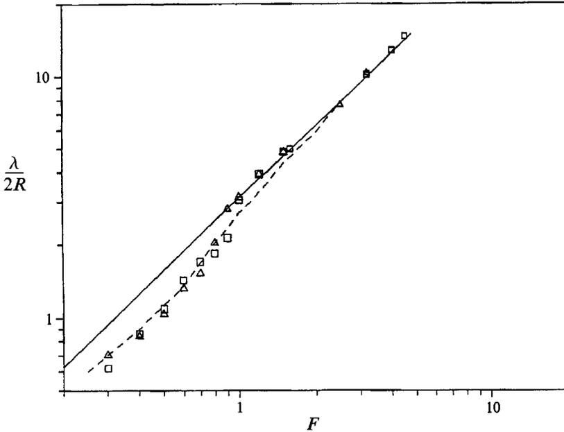
FIGURE 10. Wavelengths non-dimensionalized by  $2R$  as a function of Froude number:  $\square$ ,  $Re(1) = 2177$ ;  $\triangle$ ,  $Re(1) = 4514$ ; —,  $\lambda/2R = \pi F$ ; - - -, Hanazaki's (1988) numerical simulations.
