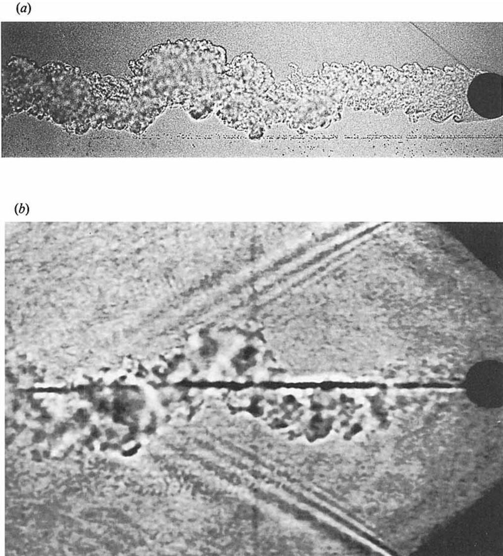
FIGURE 9. Shadowgraph visualizations of the wake for  $F > 4.5$  ( $Re(1) = 1354$ ): (a) side view,  $F = 20/\pi$ ; (b) top view,  $F = 30/\pi$  (waves on the free surface of the tank perturb the visualization from above).
