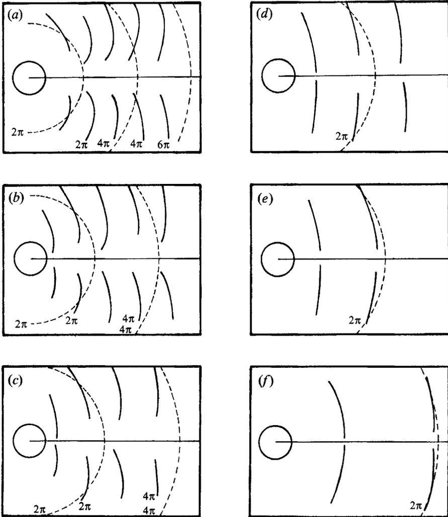
FIGURE 12. Lee wave isophases in the vertical central plane for  $Re(1) = 2177$ . —, experiments (every  $\pi$ ); ---, linear theory (every  $2\pi$ ). (a)  $F = 0.5$ ; (b)  $F = 0.6$ ; (c)  $F = 0.7$ ; (d)  $F = 0.9$ ; (e)  $F = 1.0$ ; (f)  $F = 1.5$ .
