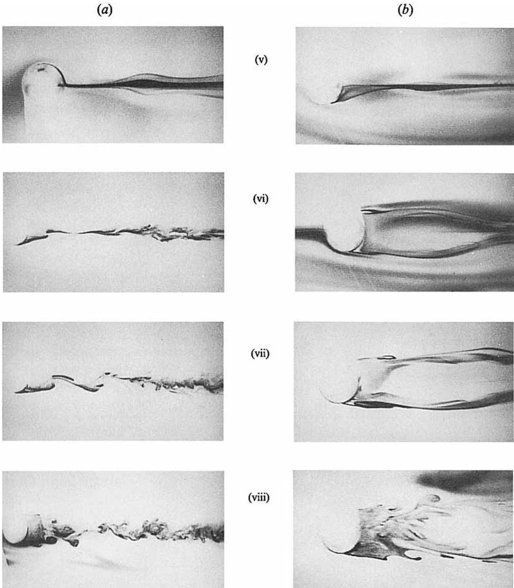
FIGURE 6. Fluorescent dye visualizations in (a) the vertical central plane, and (b) the horizontal central plane, for  $Re(1) = 329$ . (i)  $F = 0.5$ ; (ii)  $F = 0.6$ ; (iii)  $F = 0.7$ ; (iv)  $F = 0.9$ ; (v)  $F = 1.0$ ; (vi)  $F = 1.5$ ; (vii)  $F = 2.0$ ; (viii)  $F = 10/\pi$ .
