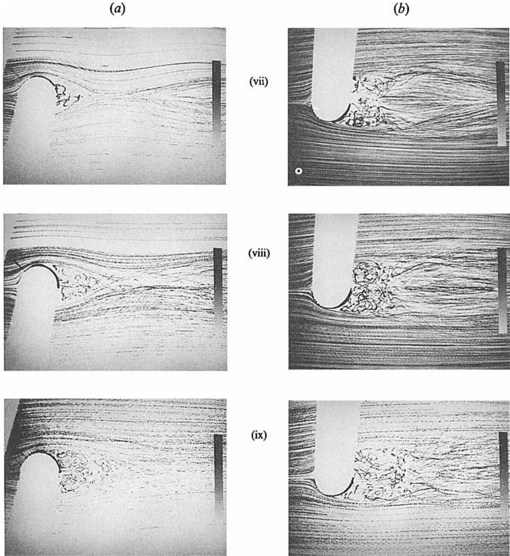
FIGURE 4. Particle streak trajectories in (a) the vertical central plane, and (b) the horizontal central plane, for  $Re(1) = 2177$ . (i)  $F = 0.4$ ; (ii)  $F = 0.5$ ; (iii)  $F = 0.6$ ; (iv)  $F = 0.7$ ; (v)  $F = 0.9$ ; (vi)  $F = 1.0$ ; (vii)  $F = 1.5$ ; (viii)  $F = 2.0$ ; (ix)  $F = 10/\pi$ .
