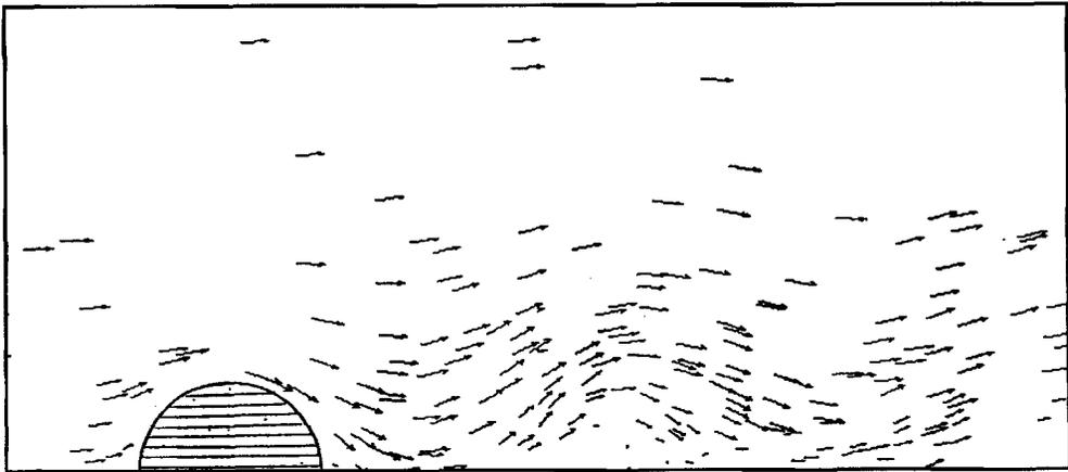
FIGURE 8. Velocity vectors relative to the sphere in the vertical central plane for  $F = 0.9$  and  $Re(1) = 2177$ .
