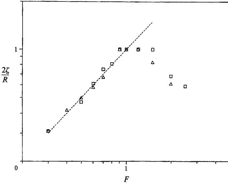
FIGURE 11. Wave amplitudes non-dimensionalized by  $\frac{1}{2}R$  as a function of Froude number.  $\square$ ,  $Re(1) = 2177$ ;  $\triangle$ ,  $Re(1) = 4514$ ; ----, Sheppard's (1956) theory.
