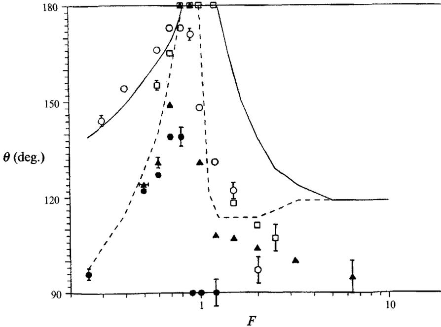
FIGURE 7. Variation with  $F$  of the separation points on the sphere in the vertical plane (open symbols) and in the horizontal plane (solid symbols).  $\square$ ,  $\blacktriangle$ ,  $Re(1) = 324$ ;  $\circ$ ,  $\bullet$ ,  $Re(1) = 1961$ . —, Hanazaki's (1988) numerical simulations in the vertical plane, ---, in the horizontal plane.
