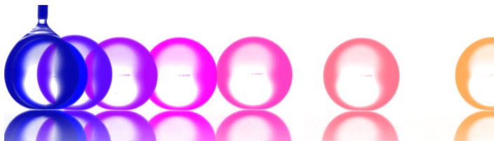
FIG. 3. Chronophotography of a millimeter-sized water droplet ( R \approx 1 mm) self-propelling on a flat reflective substrate heated at 300 °C. Water, initially immobilized by a needle located at a distance H above the substrate, detaches at a radius R \approx H/2 and then spontaneously moves away in the direction set by the internal rotation. The color gradient is used to highlight the successive positions of the drop (time interval of \approx 180 ms).
